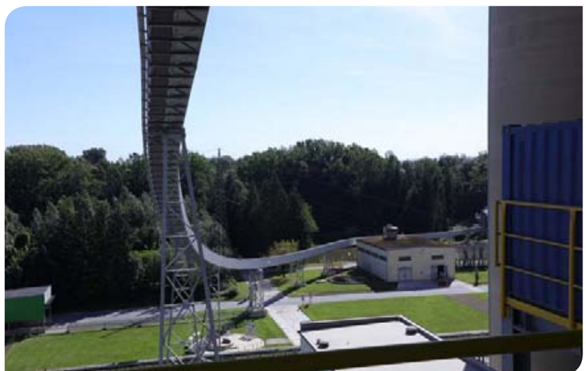
Below: Tighter curve radii than a troughed belt conveyor and higher mass flows than a pipe conveyor can be realised using a U-shape conveyor.
