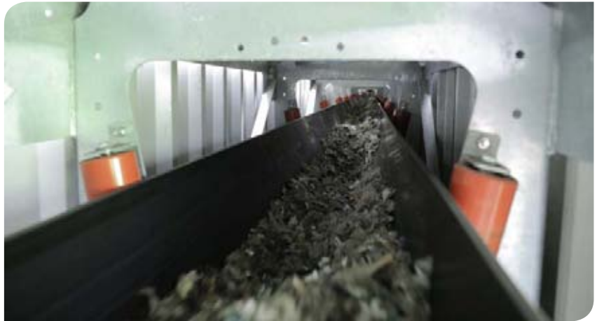
Above: Idlers form the belt into a U-shape.
